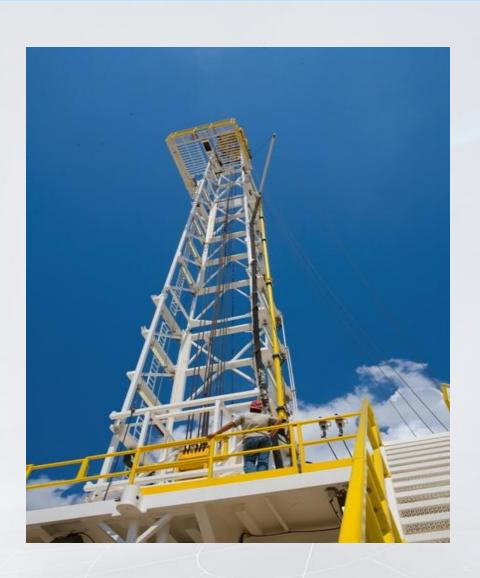
The Quicksilver® Highboy is a fit-for-purpose 1600 HP, 750,000 lbs static hook load, Hydraulically raised triples mast with a 26-foot substructure designed for a larger BOP if required.
